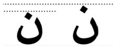
Figure 2. Example of vertical displacement of the point in an Arabic letter to hide a bit value
